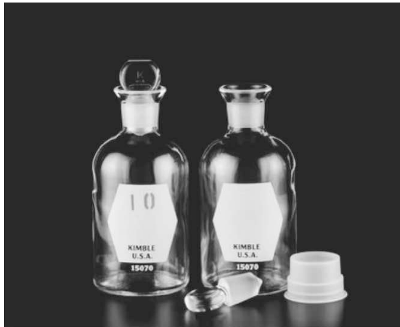
Figure 11.5 Bottles specifically designed for incubation of water samples for BOD analysis. A flared mouth forms a water seal which prevents the drawing of air into the bottle during incubation. The interior shape of the bottle is such that the entrained air is swept out of the stopper opening. Glass stopper design uses a conical extension to displace excess sample which further insures no air entrapment in the sample. (Krackeler Scientific, Inc.).
