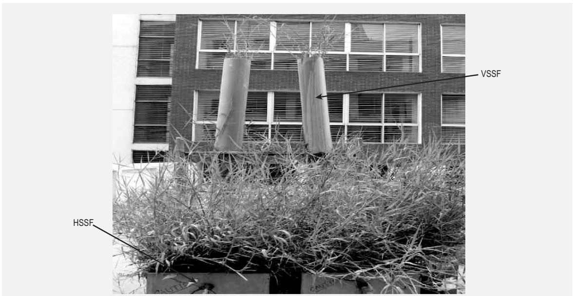
Figure 8.11 Arrangement of lab-scale wetland systems for textile wastewater treatment.
